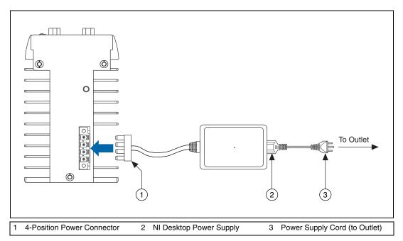
Figure 2-3. Wiring Power to the CVS-1450 Device
